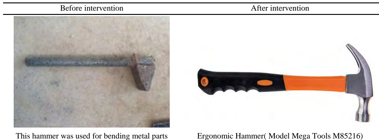
Figure1: Hammer, Left side: Old design, Right side: Ergonomic design
